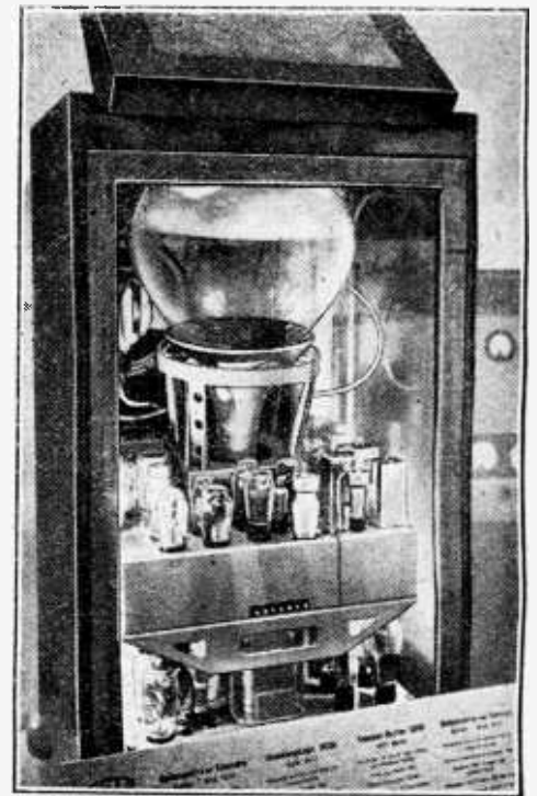
TELEVISION IN ITALY. The latest large tube cathode-ray television receiver shown by the "SAFAR" Company at the ninth annual wireless show held in the Triennial Palace, in Milan.
