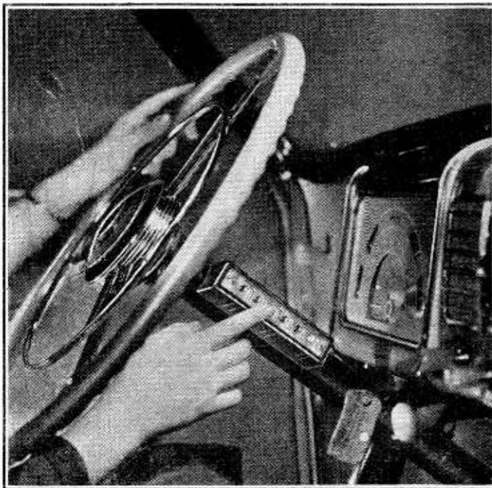
AUTOMATIC TUNING FOR CAR RADIO. With the help of this control panel, any one of five stations may be tuned-in instantaneously by pressing the appropriate button. An associated unit, measuring 2\frac{1}{2} \times 4\frac{1}{2} \times 4\frac{1}{2} ins, is clamped to the side of the receiver. By pressing the "off" button, the normal manual tuning system comes into operation. The control system, which has been introduced by an American firm, is stated to be applicable to any car set; its use is claimed to make for greater safety on the road.
