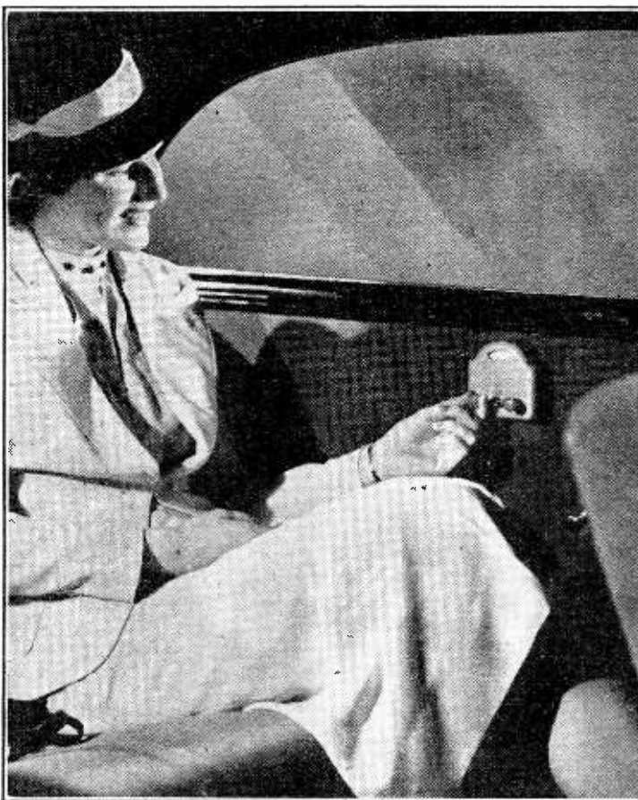
BACK-SEAT CAR RADIO. With this mechanically operated remote-control attachment, passengers in the rear seats can control the usual type of dashboard-mounted car radio set. The receiver can be operated at will from either the normal or remote control points; both indicating dials register the same reading. The unit, developed in America, is applicable to most makes of set.
